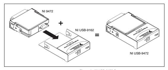
Figure 1. NI USB-9472 Components
